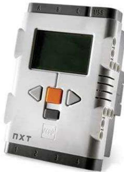
Figura 1 - NTX Intelligent Brick, bloco central do robô
